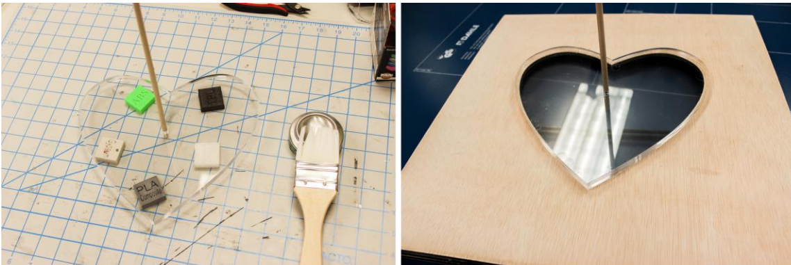
Figure 17 Light assembly built with 5mm Acrylic sheet
